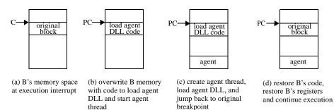
Fig. 3. "Code Patching" an Agent into Binary B
