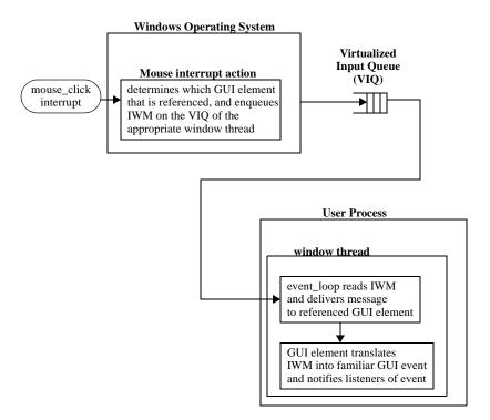
Fig. 4. Translation of Mouse Inputs into GUI Events
