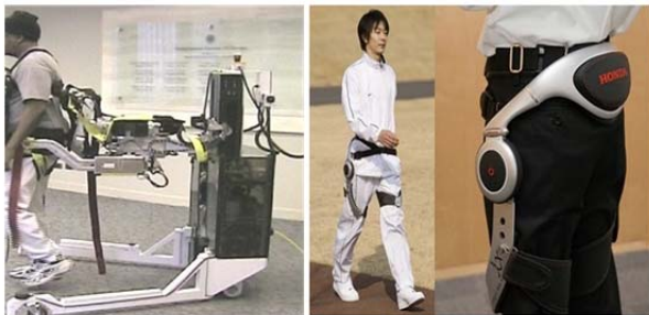
Fig. 6. Left: KineAssist used for standing balance, ambulation and dynamic balance therapy allows therapists to focus on useful tasks with reduced fear of falls. Right: Honda Stride Management Assist device. For those with weakened leg muscles who are still able to walk.
