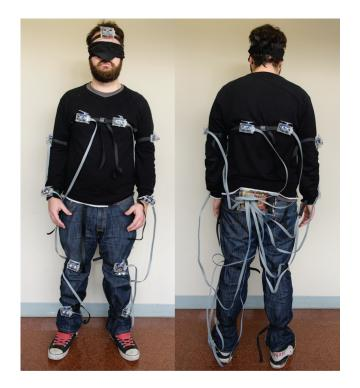
Figure 1: SpiderSense on a blindfolded user
