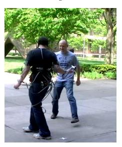
Figure 11: The wearer sensing one of the experimenters approaching from behind and throwing a cardboard shuriken.
