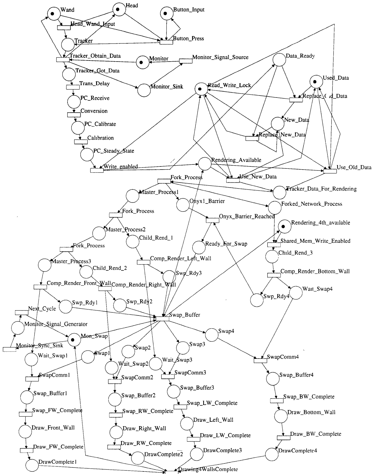
Figure 1: Time Petri net model of the CAVE virtual environment.
