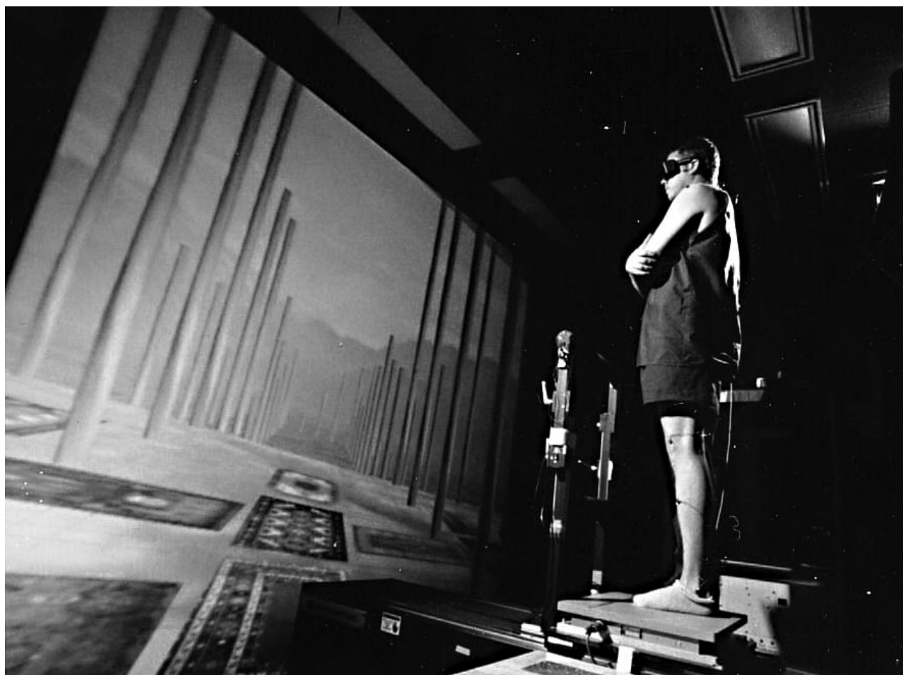
FIG. 1. Dynamic image presented in the VEPO laboratory to a subject standing on the translating sled. Subject is wearing shutter glasses (Crystal Eyes; StereoGraphics Inc.) in order to perceive the stereo image.
