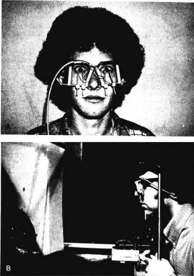
FIG. 1. A, eye movement monitor with binocular photocell sensors mounted on a modified ophthalmic frame in place on patient. Circular photocells positioned approximately 12 mm from the eye and perpendicular to the globe measure amount of infrared light reflected from the nasal or temporal limbus, respectively. B, patient's head supported by headrest and chinrest. The target is a small spot of light moving on a large, translucent screen 57 cm away (on left). Infrared light source (lower left) is a tungsten lamp with a Kodak No. 2 darkroom safelight filter.
