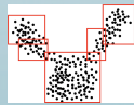
Figure 1: CHDR covering a non-convex geometric object. [from B. J. Gao and M. Ester, "Turning clusters into patterns: Rectangle-based discriminative data description," in ICDM 2006]
