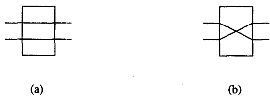
Figure 2.11 Two switching configurations of the 2 \times 2 switch: (a) Pass-through; (b) Cross-over. Copyright (r) 1994 Benjamin/Cummings Publishing Co.
