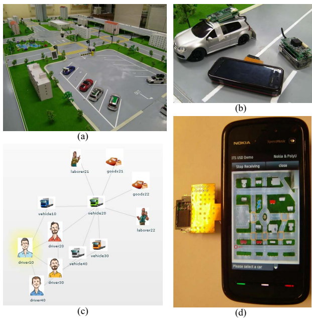
Figure 7. (a) Snapshot of our Smart Traffic System testbed, (b) Smart car, smart phone with uSD card, and sensor mote, (c) Context map for the logistic application, (d) Logistic vehicle tracking (using an area map of the testbed) through the mobile phone (vehicle shown with red circle and arrow)
