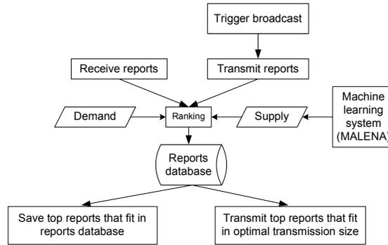
Figure 2.1. Principles of the TrafficInfo algorithm (execution at an individual vehicle)
