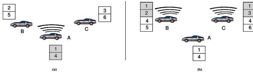
Figure 1.1. Rank-based store-and-forward. (a) Vehicle A broadcasts its top two reports which are reports 1 and 4. (b) After receiving from A, vehicle B incorporates the received reports, re-ranks, and broadcasts the top two (shadowed). The same for C.
