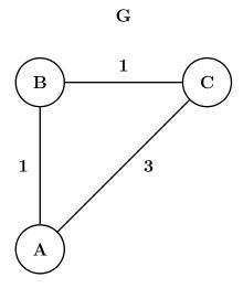
The shortest path between A and C is A-B-C of total weight 2
