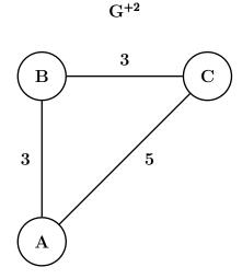
The shortest path between A and C is A-C of total weight 5
