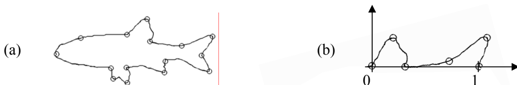
Figure 1. (a) Key points are positive local maxima and negative local minima of curvature. (b) An example of a normalized part (from front of dorsal fin to center notch of tail).
