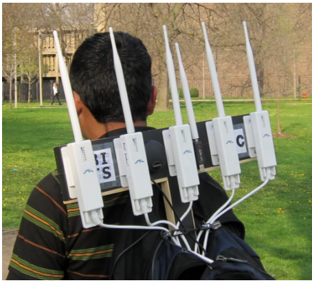
(a) Mobile monitor carried in a backpack. The mobile node includes 5 synchronized Wi-Fi radios, a spectrum analyzer, and a GPS receiver.
