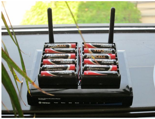
(b) Stationary monitor with a 24h battery pack. Stationary monitors upload traces to mobile management consoles, avoiding the need for a reliable backhaul connection.
