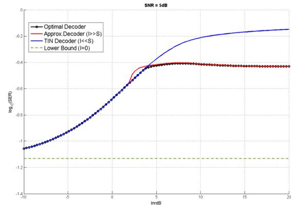
Fig. 2: BER for 4QAM with SNR=5 dB vs INR in dB.
