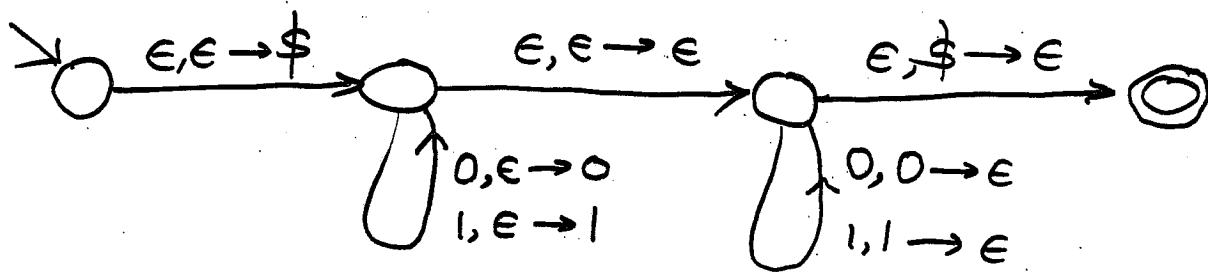
$N\text{-PDA} \longleftrightarrow CFG \longleftrightarrow CFL$
