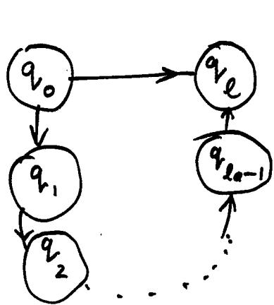
read 'a', pop 's', push  $\underbrace{u_1 u_2 u_3 \dots u_l}_{\text{R.H.S. of a rule.}}$
