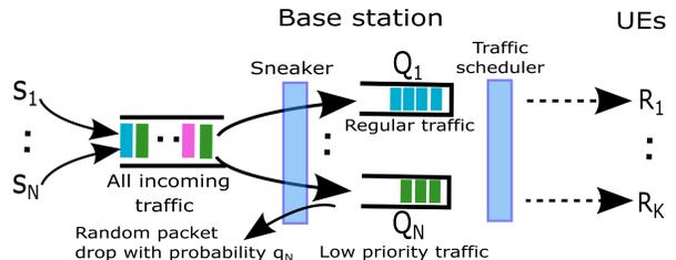
Figure 2: Example cellular system setup with *Sneaker*
