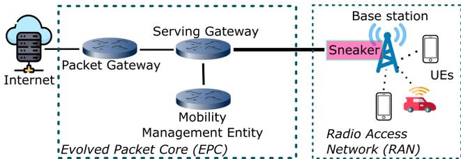
Figure 1: The service architecture in LTE network
