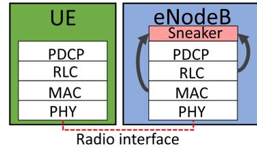
Figure 3: LTE protocol stack
