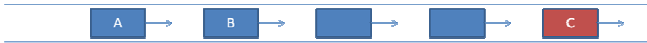
Figure 1. Assumed scenario for deriving the formula. Shows vehicle C sending report to vehicle A, which has vehicle B in front of it.
