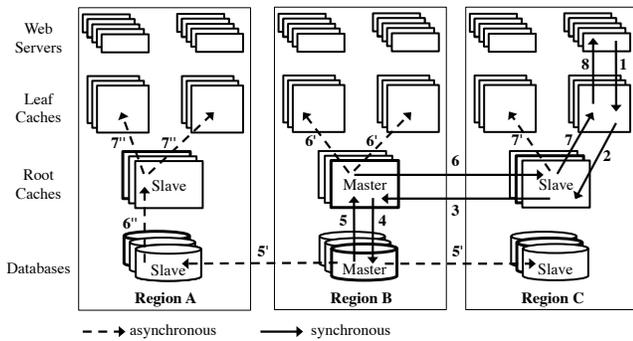
**Figure 1: The write path for Facebook’s replicated storage. On-path caches are synchronously updated; off-path caches are asynchronously invalidated. There is a single master region for each shard with the root-master cache and master database. Different shards may have masters in different regions.**
