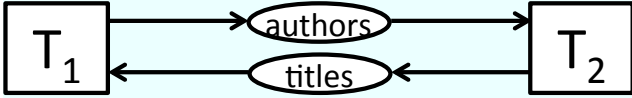
Figure 1: A lock graph for the transactions shown in Table 1. The lock graph shows the hold-and-wait cycle T_1 \rightarrow \text{authors} \rightarrow T_2 \rightarrow \text{titles} \rightarrow T_1 .
