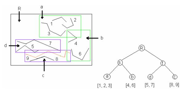
Fig. 1.b – After the insertion of the trajectory 9 in 2D R-tree In the above illustration, the MAXLEAFSIZE is 3
