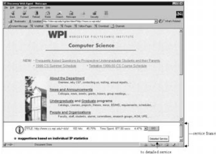
Figure 1 The WebSA interface, as provided by a separate frame at the bottom of a browser page.
