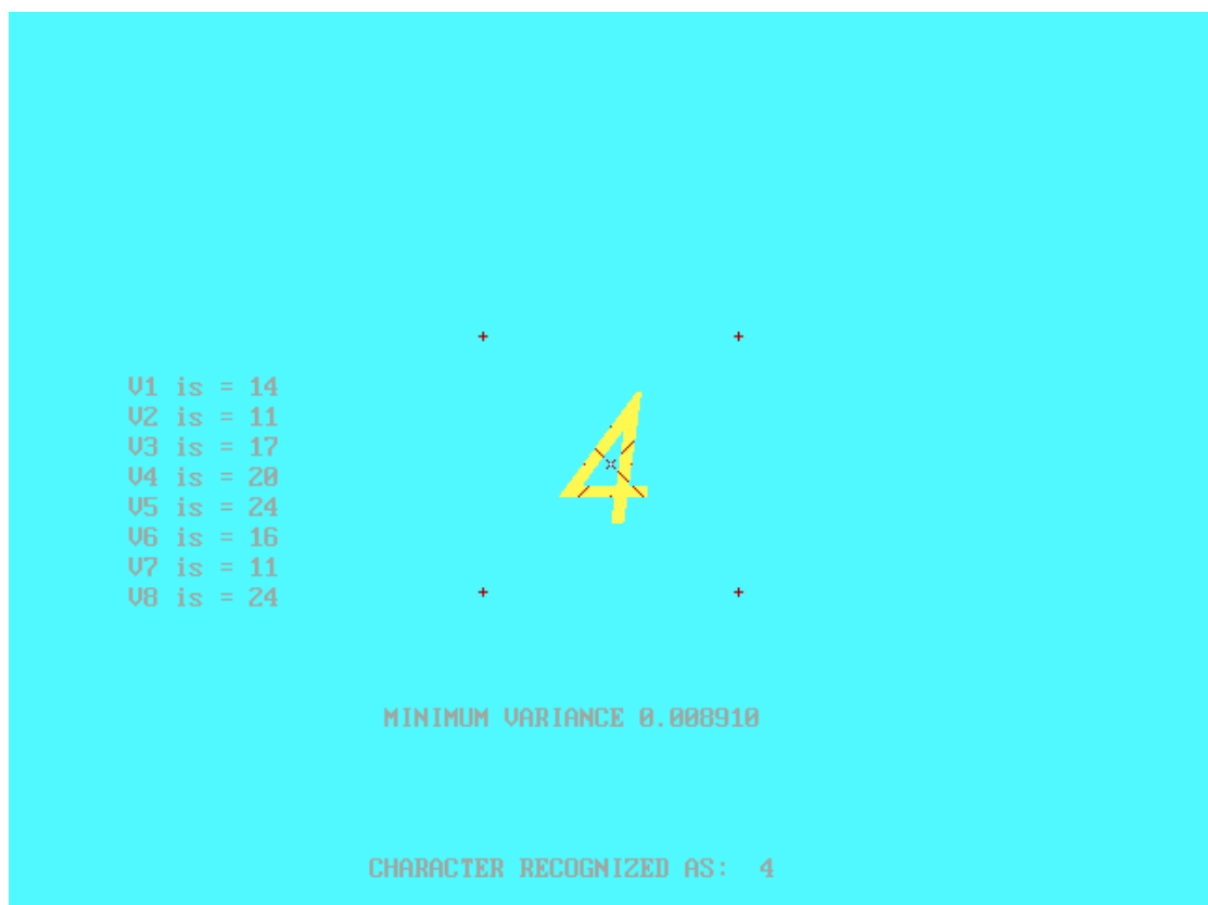
FIG 16 :CALCULATING VARIANCE AND DISPLAYING RECOGNITION RESULTS.
