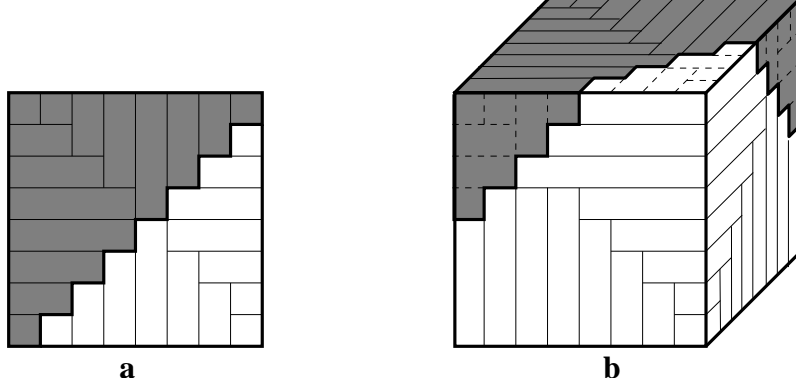
Figure 8: The pattern created by the algorithm in (a) two and (b) three dimensions. The shaded part is filled with the herringbone arrangement for minima sequence, the other half is filled with the arrangement for maxima sequence.
