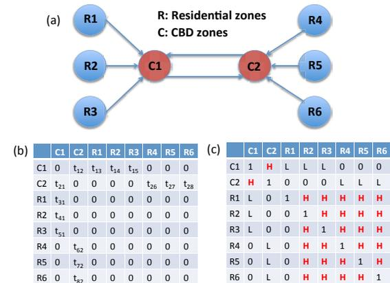
Figure 1: Concept: Predicting similarity structure by correlations: (a) Traffic flow between residential and CBD zones. (b) The traditional trip distribution matrix. (c) Dense zonal traffic flow (time-series) correlation based structure; H = High, L = Low. Static trip distributions do not capture high level similarity between traffic characteristics of zones. In this paper, the dynamic sparse optimal structure of the dense (c) is inferred in real time, for arbitrary temporal granularity.
